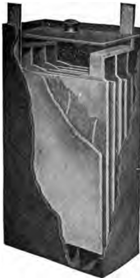
FIG. 317.—One Cell of the "Gould" Storage Battery for Electric Vehicle Use. According to the data given by the manufacturers, this cell, containing four negatives and three positive plates, has a normal charging rate of 27 amperes; a distance rate of 22\frac{1}{2} amperes for 4 hours; a capacity of 81 ampere-hours at 3 hours' discharge, and of 90 ampere-hours at 4 hours' discharge. The plates are each 5\frac{1}{2} \times 7\frac{3}{4} inches, and the total dimensions of the cell, enclosed in its rubber jar, are 2\frac{1}{2} \times 6\frac{1}{4} \times 11 inches. Forty such cells are generally used for an average light vehicle battery.
